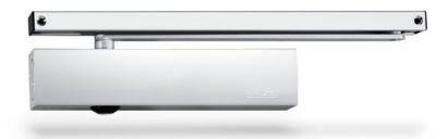
Opposite hinge side overhead door closer with guide rail for single-leaf doors up to 1400 mm leaf width with latching action and brake-to-stop function
